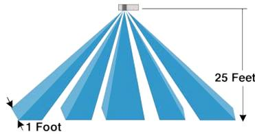
The area of width coverage is variable by distance between the sensor and the object being monitored, the closer "narrow" the further "wider". Also, the segments shown can be masked "off", with tape, allowing coverage to just the exact area desired.
